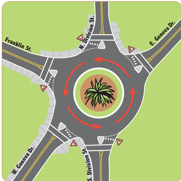
Continuous counterclockwise traffic flow
