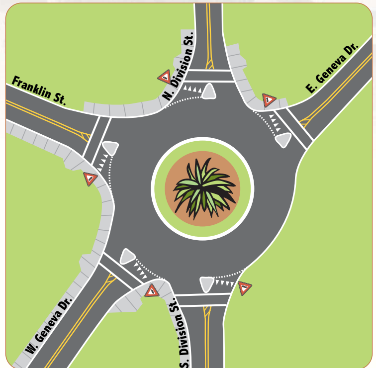
Conceptual drawing of the 5-leg roundabout at Franklin St., Geneva Dr. and Division St.
